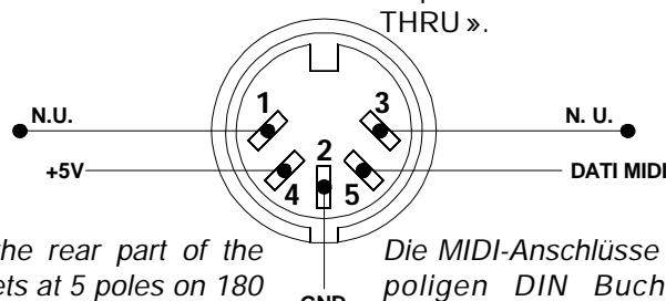
*The MIDI connectors situated on the rear part of the equipment are supplied of DIN sockets at 5 poles on 180 degrees in compliance to the international standards.*
